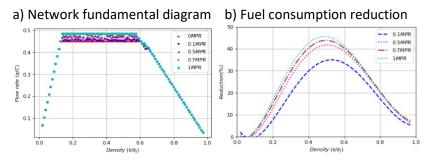
4. The capacity and the fuel consumption reduction with different ASL implementation areas based on the Krauss model are shown below. We recommend the ASL implementation area to be about 100m, which can guarantee control results as well as reduce computation costs.
